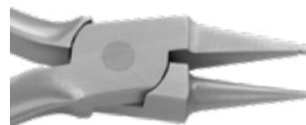
Light Wire Bird Beak Pliers w/ Groove A longer cone than a standard bird beak is useful for forming precise loops in light wire. The groove allows for locating and duplicating loops. <= .020" (.51mm) 678-305
