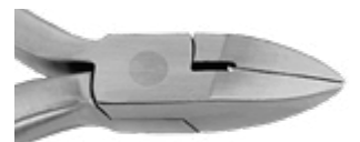
Micro Mini Ligature Cutter, 15° 15° offset tip with ultra slim profile is a plus in the most difficult to access areas. Designed to cut soft wire pins and ligature wires. <= .012" (.30 mm) 678-109
