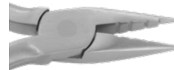
Jarabak Pliers Versatile light wire bending pliers. Grooves assist with precise bending and closing of loops. Serrated surface grips wires. <= .020" (.51mm) 678-301
