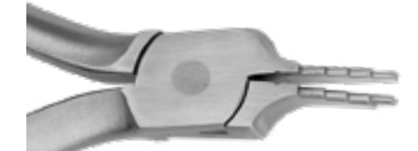
Nance Loop Forming Pliers For precise forming of loops in four lengths: 3, 4, 5 and 6 mm. Groove at base aids in closing loops. <= .022" (.53mm) 678-319
