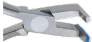
Slim Flush Cut & Hold Distal Cutter, O-Ring Style Cuts and holds wire distally flush to the buccal tube while reducing debondings. The slim design also helps to improve intraoral visibility. Replaceable blue silicone ring holds the cut wire until released. <= .012" to .021" x .025" (.30 mm — .53 mm x .64 mm) 678-114
