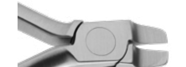
Slim Arch Bending Pliers Designed for placing first, second and third order bends. .025" blade width. <= .022" x .028" (.56mm x .71mm) 678-307S
