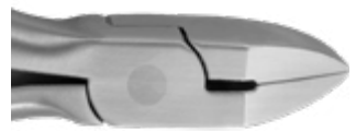
Hard Wire Cutter, 15° 15° offset tip enhances access in difficult areas. Designed to cut hard wires. <= .022" x .028" (.56 mm x .71 mm) 678-103
