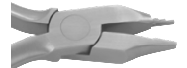
Tweed Loop Forming Pliers Loop forming pliers with .055", .075" and .090" diameters for creating bull and helical loops in wires. <= .022" x .028" (.56mm x .71mm) 678-306
