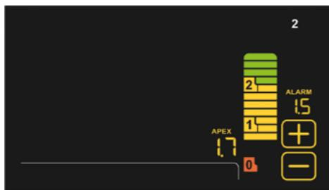
**Apex locator.** The apex distance is displayed on the LCD during the root canal instrumentation phase. The nearing of the apex is verified by the ENDO software. Once the apex is reached the Apex-Stop function interrupts micromotor rotation.
