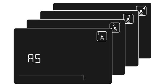
**Multi-profile feature.** Cuspidor-cup system automatisms, favourite working positions and settings for every single instrument can be saved for up to 4 different users, ensuring maximum versatility of use. This function is useful in multi-dentist surgeries or in clinics where there is high turnover of specialists.
